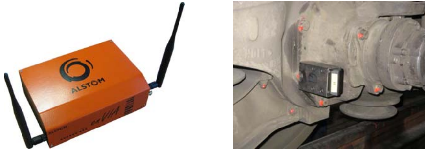
Figure 2: Gateway and mote (attached to a bogie) of use with the CBM OB.
